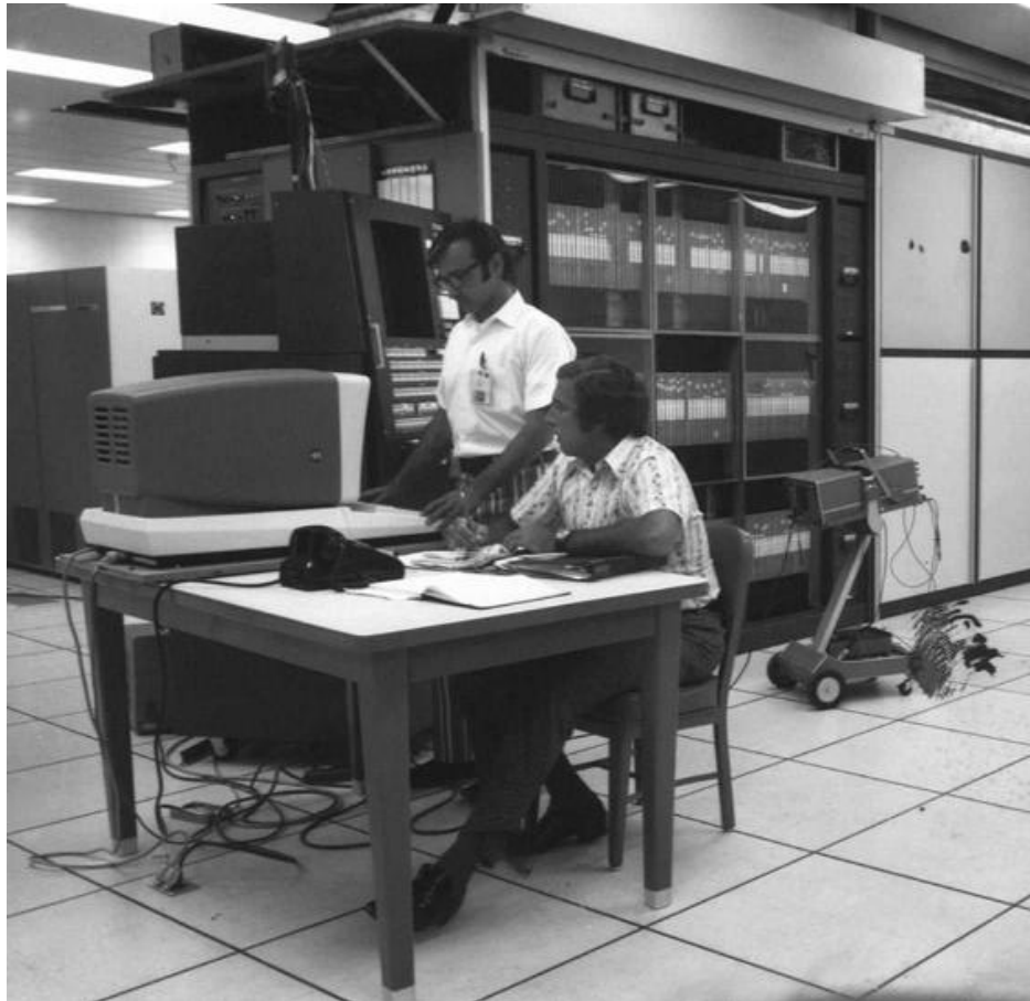
FIGURE E6.16.1 The Illiac IV control unit followed by its 64 processing elements.
