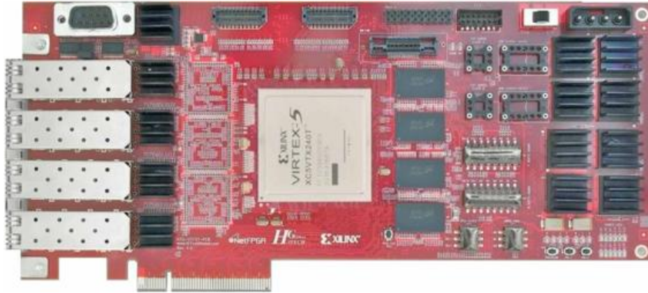
FIGURE E6.10.1 The NetFPGA 10-Gigabit Ethernet card (see http://netfpga.org/ ), which connects up to four 10-Gigabit/sec Ethernet links. It is an FPGA-based open platform for network research and classroom experimentation.
