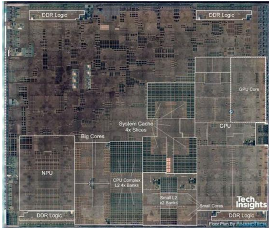
FIGURE 1.9 The processor integrated circuit inside the A12 package. The size of chip is 8.4 by 9.91 mm, and it was manufactured originally in a 7-nm process (see Section 1.5 ). It has two identical ARM big processors or cores in the lower middle of the chip, four small cores on the lower right of the chip, a graphical processor unit (GPU) on the far right (see Section 6.6 ), and a domain-specific accelerator for neural networks (see Section 6.7 ), called the NPU, on the far left. In the middle are second-level cache memories (L2) for the big and small cores (see Chapter 5 ). At the top and bottom of the chip are interfaces to main memory (DDR DRAM). (Courtesy TechInsights, www.techinsights.com , and AnandTech, www.anandtech.com )
