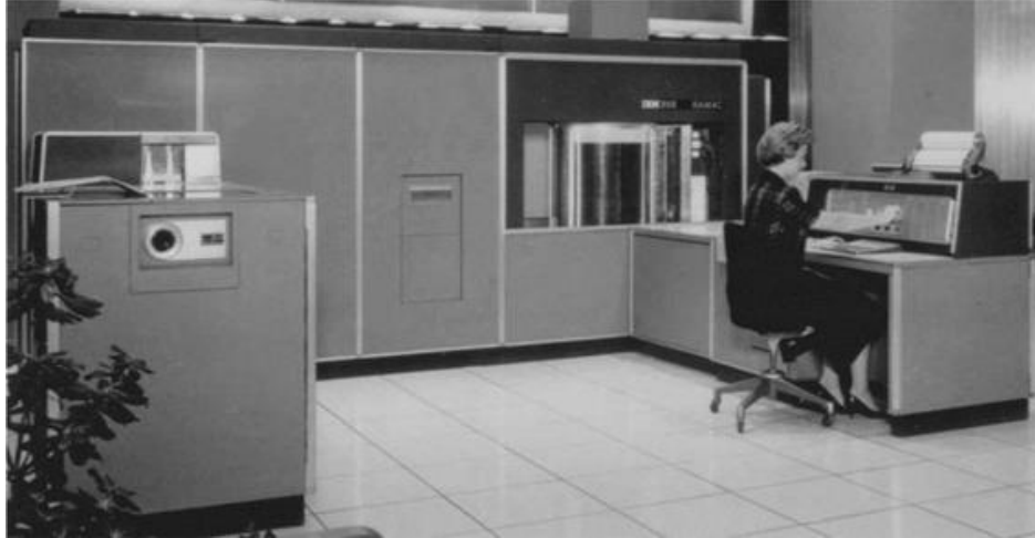
FIGURE E5.17.6 The RAMAC disk drive from IBM, made in 1956, was the first disk drive with a moving head and the first with multiple platters.
